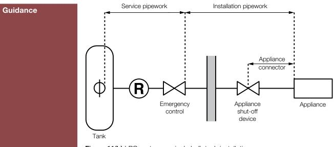
Figure 11(b) LPG systems - single bulk tank installation (Note: Some vapour installations may have an additional regulator)
