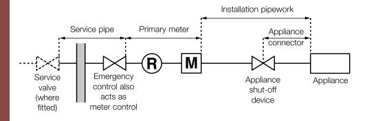
Figure 6 Inside meter installation
