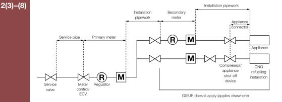
Figure 4 Single supply with two secondary meters
